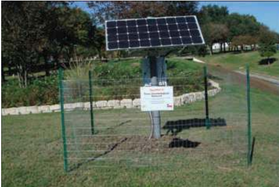
◀ TexNet seismometers placed throughout the state, like this one in Dallas, monitor seismic activity across Texas. Courtesy The University of Texas at Austin Bureau of Economic Geology
