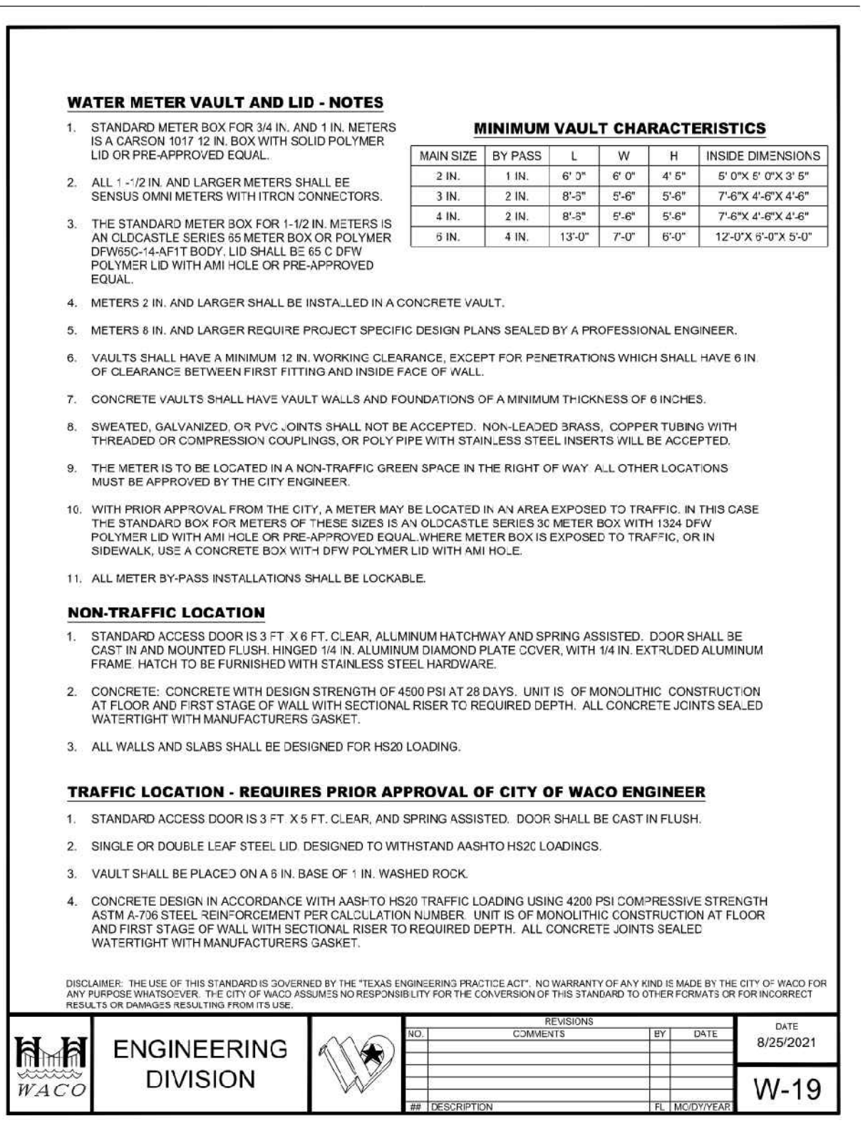
C5 WATER METER VAULT & LID NOTES N.T.S.
