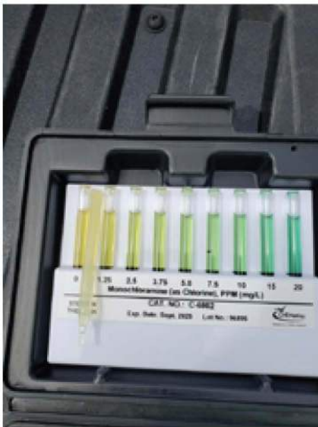
Field sampling for monochloramines in the groundwater at a Florida landfill.
