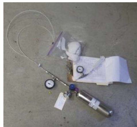
Collection of soil vapor sample using Summa canister. (photo courtesy SCS Engineers)
